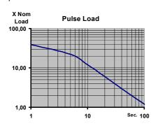
The curves show the pulse load ability compared to the nominal load for the CDH resistors under the following conditions: The load is a periodic pulse load with a constant **period time** of **120 sec**
