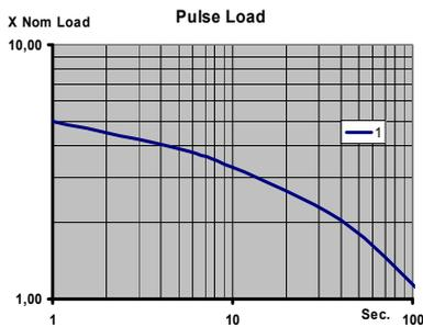
For further optimization DANOTHERM offers individual thermal electric circuit models for all types and ohm values. With these models the temperature of the resistor wire during any pulse load conditions can be simulated with a standard soft ware like P-Spice. Alternatively Danotherm offers to make thermal simulation for our customers
