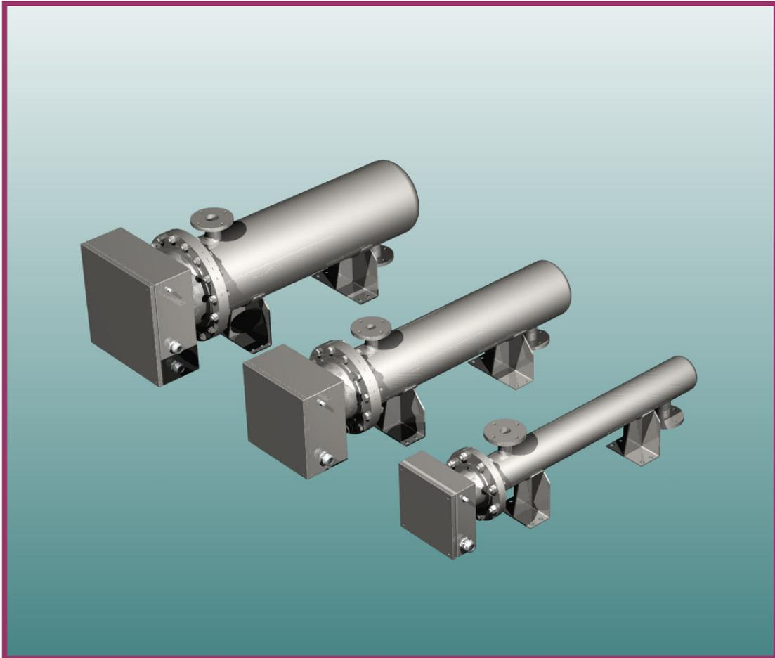
**V14-150-08, V14-250-16 and V14-350-28** is a range of water cooled high power brake resistors. The resistors consist of stainless steel tube resistors with diameter 14 mm and length 2200mm (V14/2200) mounted in stainless (AISI 304 or AISI 316) water tanks. The electrical connections complies to protection class IP 00 to IP 65 according to customer specifications
