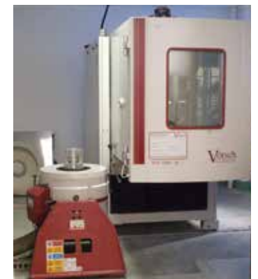
Test equipment combines vibration together with environmental and electrical test.
